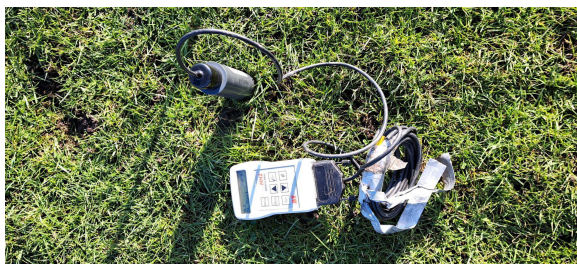
Fig. 3 The Thetaprobe standard set from Eijkelkamp
